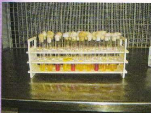
Sugar (sucrose) fermentation test for E. coli isolates, red: negative, yellow: positive
