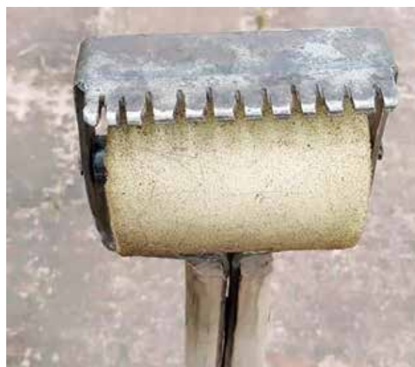
Sponge roll and comb of Manual Ectoparasite Expeller cum drug applicator
