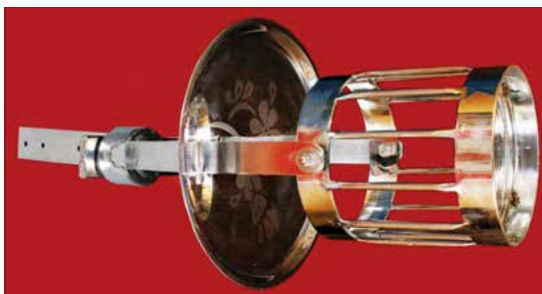
Figure 9: Side view of the Desave Mineral block Dispenser for Mithun, Cattle and Buffalo
