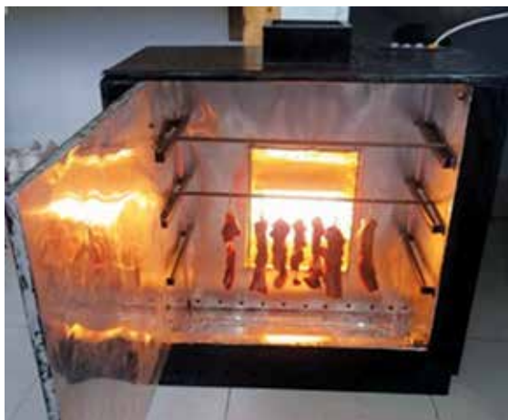
Figure 6: Inside view of the Innovative Meat Dryer
