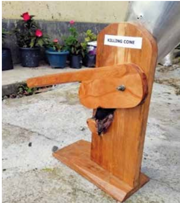
Figure 31: Right side view of innovative chicken killing cone
