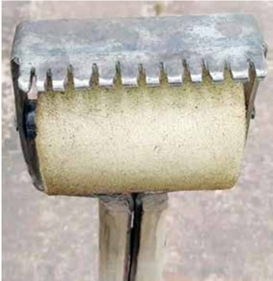
Figure 1: Head of the Large Animal Ectoparasite Expeller cum Drug Applicator
